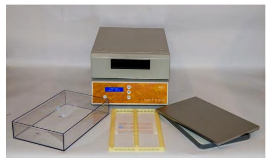
FIGURE 14. HybEZ™ II Hybridization System
